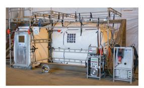
The WICH System is a patented, versatile, customisable system that is designed to facilitate hot work such as welding in hazardous areas offshore or onshore.
