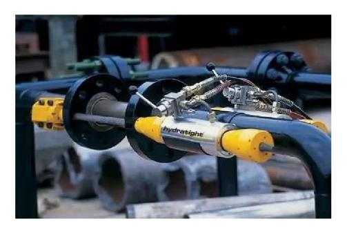
Flange puller services are used to exctract flanges or heat exchanger tube bundles prior to commencing with cleaning operations or replacing the tubes with the new ones. We undertand that bundle pulling is a delicate process which requires precision and AWI are equipped with best equipment and highly trained personnel to perform the service at the highest standard.
