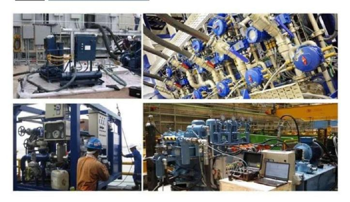
Flushing is a process which is done to clear any contaminants present in the pipe and oil after installation. The sole purpose of this process is to avoid damage caused by contaminants/dirt's to the end using equipment. The pipes are cleaned by creating a turbulent flow in the system and passing them through filters until the desired cleanliness value is obtained.
